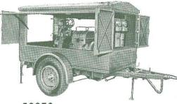
Mobile power plant comprising: 1-S-108 model engine, 15 B.H.P. at 1,500 r.p.m. and 10 kVA alternator with switch panel.
